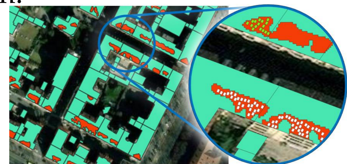
Fig 3. Optimal cross-roof PV placement
