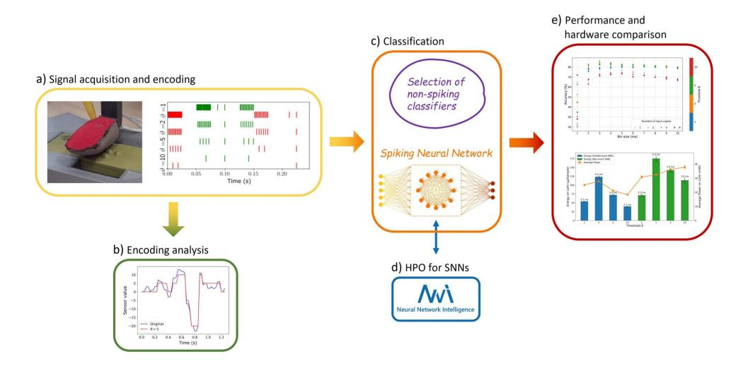
This neuromorphic pipeline for reading Braille letters with a digital sensor is a proof time-varying pattern for concept of recognition in edge applications with neuromorphic hardware. The digital sensor data requires encoding into the spike domain; the network runs on Intel Loihi.
